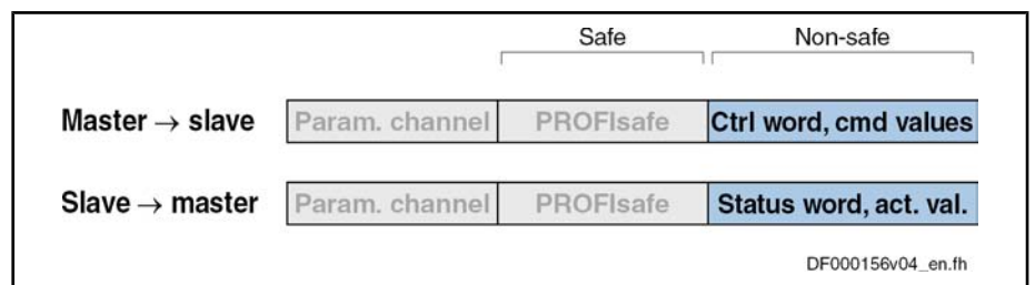
Fig.4-52: Position of the Non-Safe Process Data Channel in the Cyclic Data Channel
