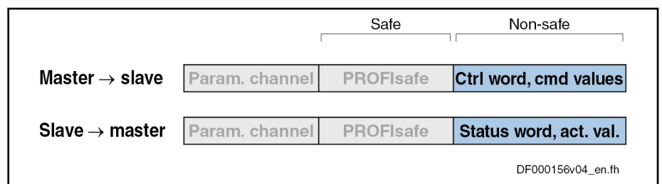
Fig. 4-40: Position of the Non-Safe Process Data Channel in the Cyclic Data Channel
