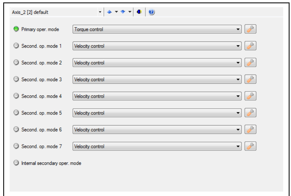
Fig. 5-5: IndraWorks dialog for setting the operation mode for the slave axis
