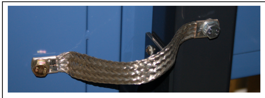
Fig. 29-4: Example of a braid wire to connect to a machine frame
